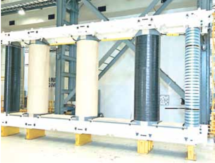
5 Limb Core of 315 MVA, 400 kV Auto Transformer
